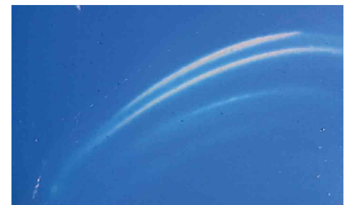
Excellent pigment stabilization "rub out test"
