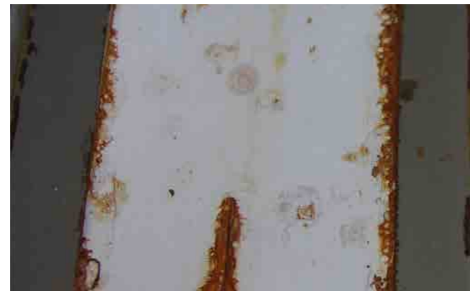
Weak corrosion protection in 2 layer system
