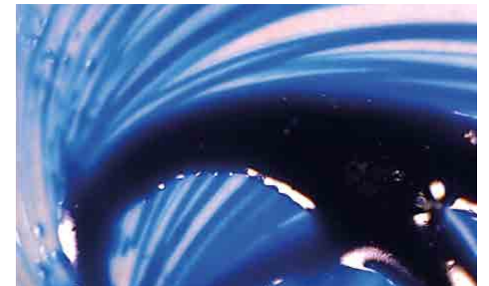
Strong pigment floating visible "rub out test"
