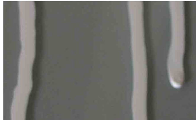
Sagging of paint on vertical substrate
