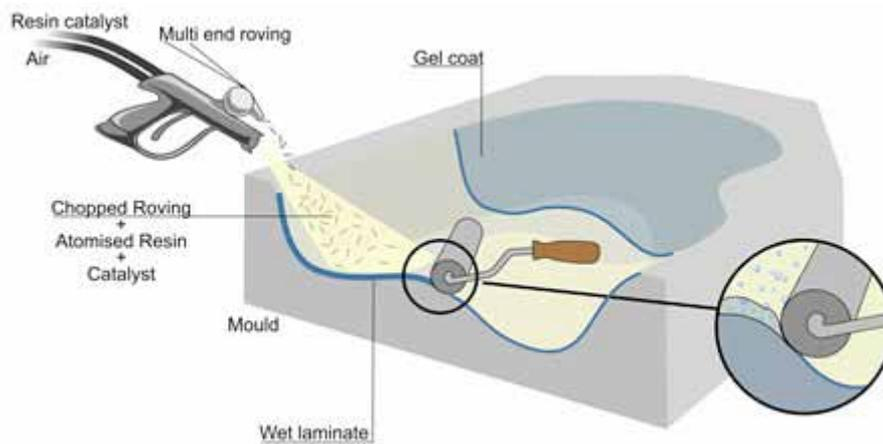
Although the process can be robotised, it generally requires skilled operators to obtain consistent high quality parts. The same low cost open moulds that are used in hand lay-up are used in spray-up application. Spray-up is primarily for polyester and vinyl ester resins and glass fibre.
