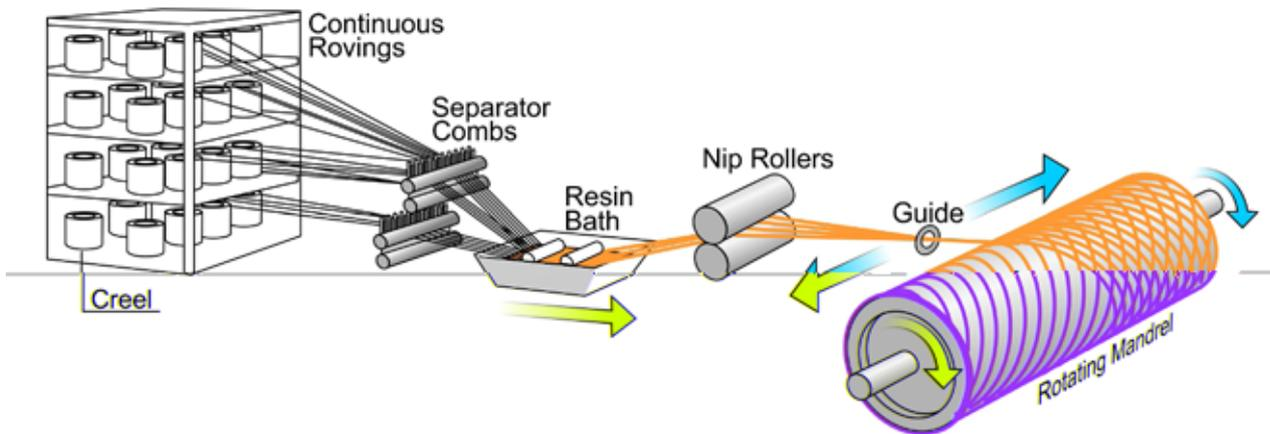
Specific mechanical properties are achieved through reinforcement and resin selection, careful fibre orientation and thickness. Suitability to operating environment is primarily determined by the resin matrix and internal lining. However reinforcement selection should also be carefully considered. Programs can adjust settings such as wind angle throughout the laminate build to optimise the properties.
