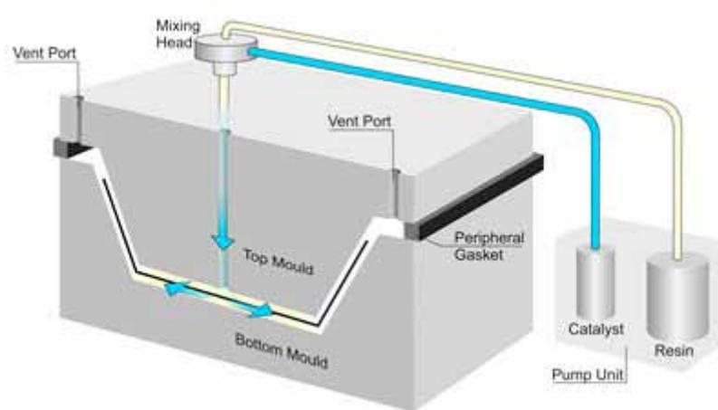
Since it can be automated and is capable of rapid production cycle times, RTM is suitable for medium to high volume production, producing relatively low cost parts. Higher production rates can be achieved by heating the moulds, using preform reinforcements and resins with short gel and cure times. RTM involves a capital investment in tooling and infrastructure that is higher than vacuum infusion but lower than compression moulding.
