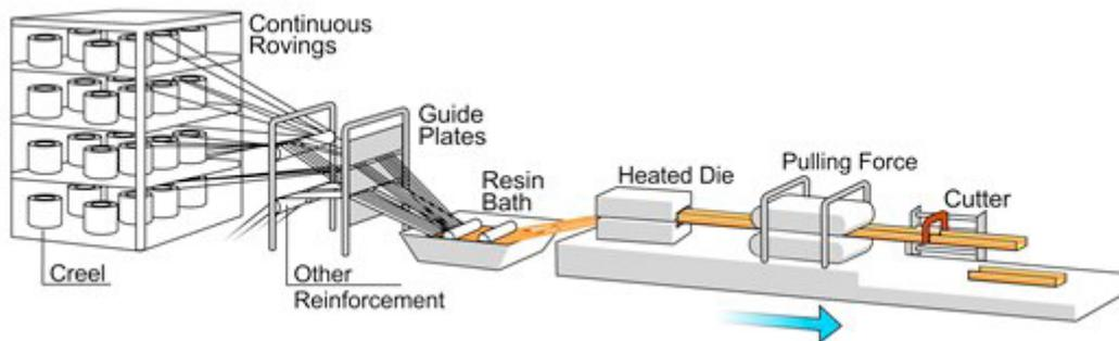
Although the mechanical properties are strongest in the machine direction (due to reinforcement fibre alignment), they can be improved in the cross wise direction by the introduction of continuous filament mat or fabrics. See also Pull Winding.
